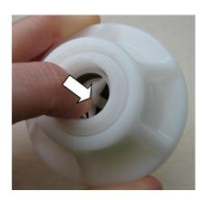
With the valve held open, submerge it in warm water with a tiny amount of washing up liquid mixed in. Move the valve backwards and forwards for a few seconds so that water is forced through the valve, removing dirt and debris. After this, flush the valve through with fresh water for one final clean.
